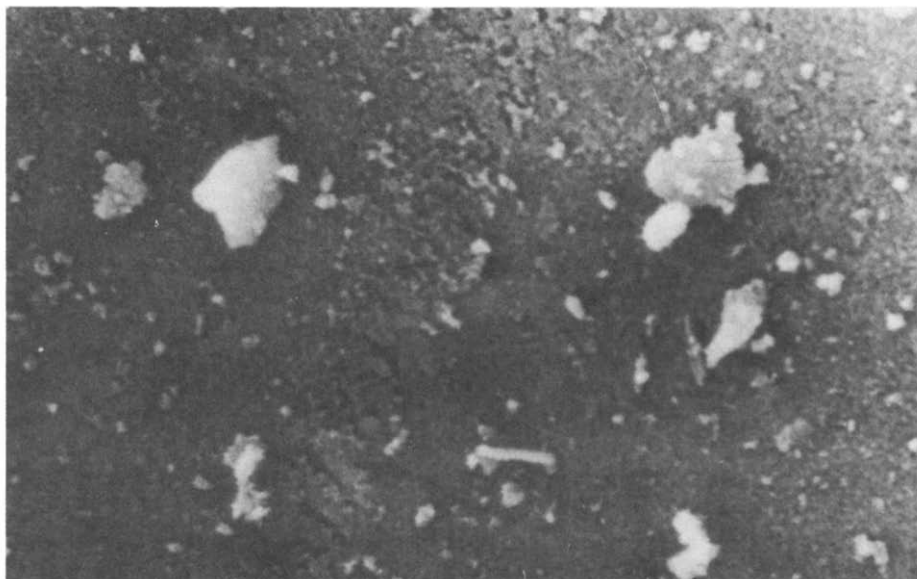
Fig. 12. Surface of Carbosil covered by a gold layer, as observed by SEM; magnification \times 1000 .
