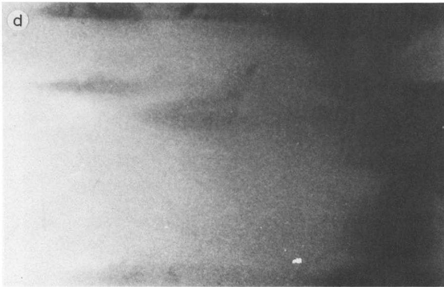
Fig. 9. Surface of the initial silica gel observed by SEM, magnification \times 1000 . A two detector system with opposite Everhart-Thornley detectors was employed. BSE = Backscattered electrons; SE = secondary electrons. a, A + B, BSE image with material contrast; b, A - B, BSE image with imaging artifacts; c, A + B, SE image with material contrast; d, A - B, SE image with topographic contrast.
